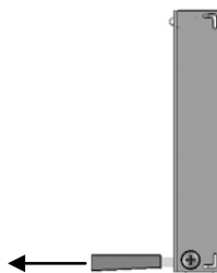
Figure 6-2: Module Handle Partially Pulled Out (Top View)
