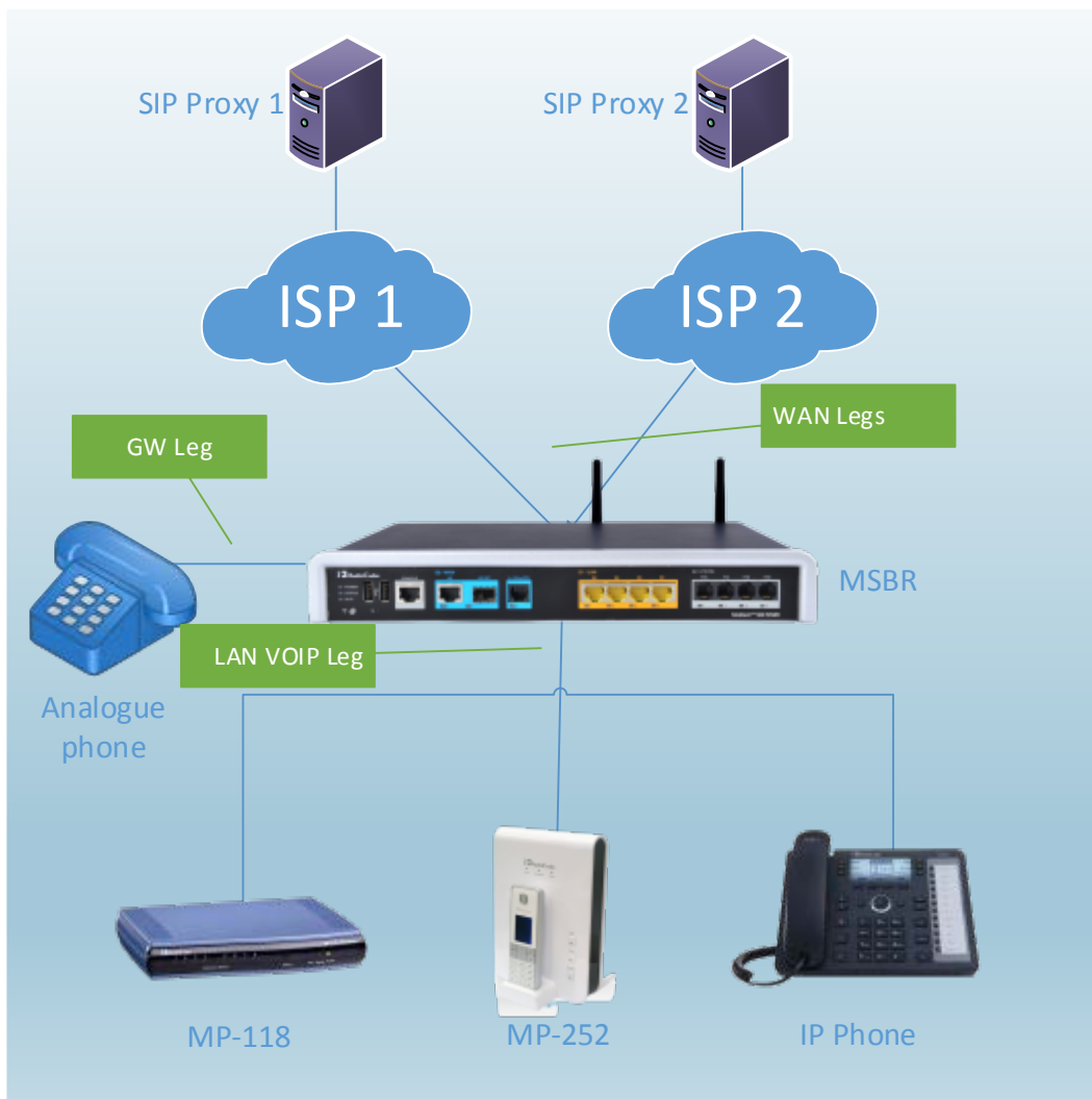
Figure 3-1: Leg Interfaces on Mediant MSBR
