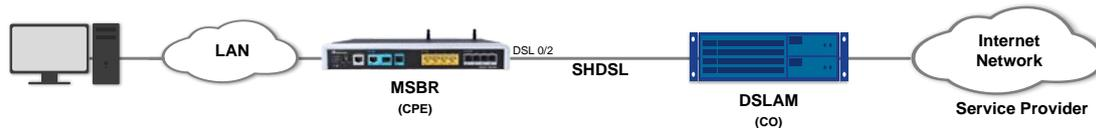
1. Configure the SHDSL interface (ATM or EFM mode):
