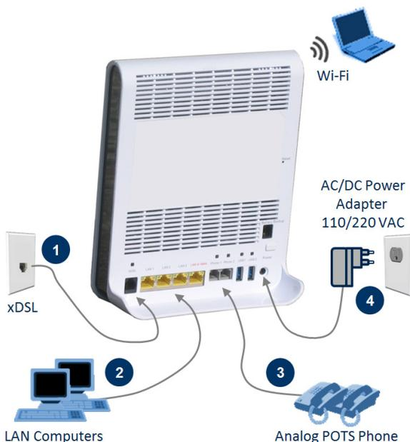
1. Connect the gateway to the Internet. If the connection type is xDSL, then connect the xDSL port to the telephone socket, using an RJ-11 telephone cable. If the connection type is WAN Ethernet, then connect the **LAN4/WAN** port to an external modem, using a CAT 5 Ethernet cable.
